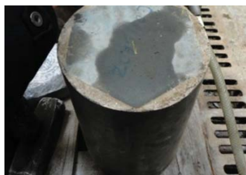
Figure 3. Typical sample in hammer test (before test)
