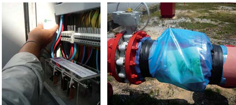
Figure 2. Coupons are experimented at field (a) Coupons placed in electrical box (b) Coupons placed at flange
